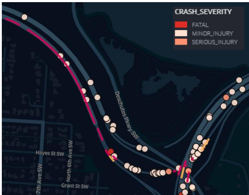
Figure 3: Weekday night speeding risk at the Highway 101 interchange with I-5 in Olympia, Thurston County overlaid with injury crash locations.
